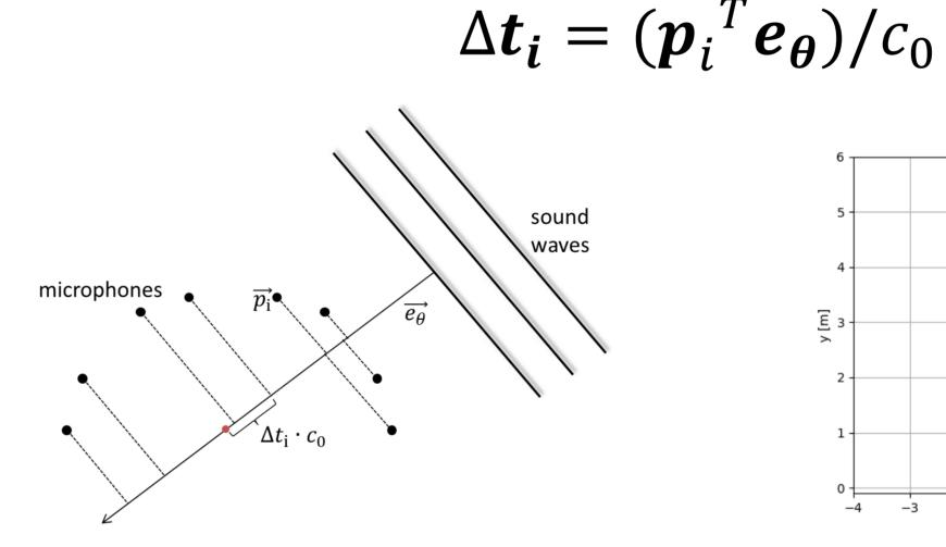
Illustration of the delay calculation for an arriving sound wave
