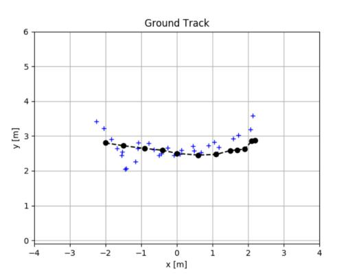
Estimated positions of a tracked person using microphone arrays
