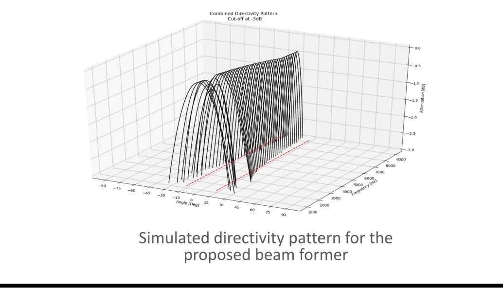
The latter one will be using the steered input from the beam former to enhance quality and robustness. We will use this to gain **voice commanding** ability.
